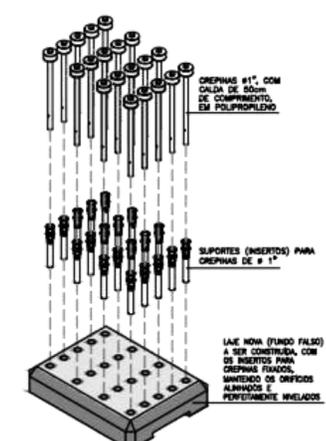
DET. MONTAGEM DAS CREPINAS Ø1" (ESQUEMÁTICO)
